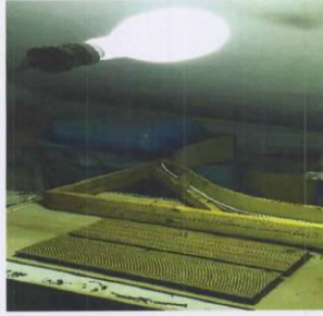
Figure 5. The artificial weathering (UV test)
