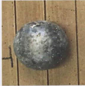
Figure 2. The Impact Strength Test (Steel Ball Test)
